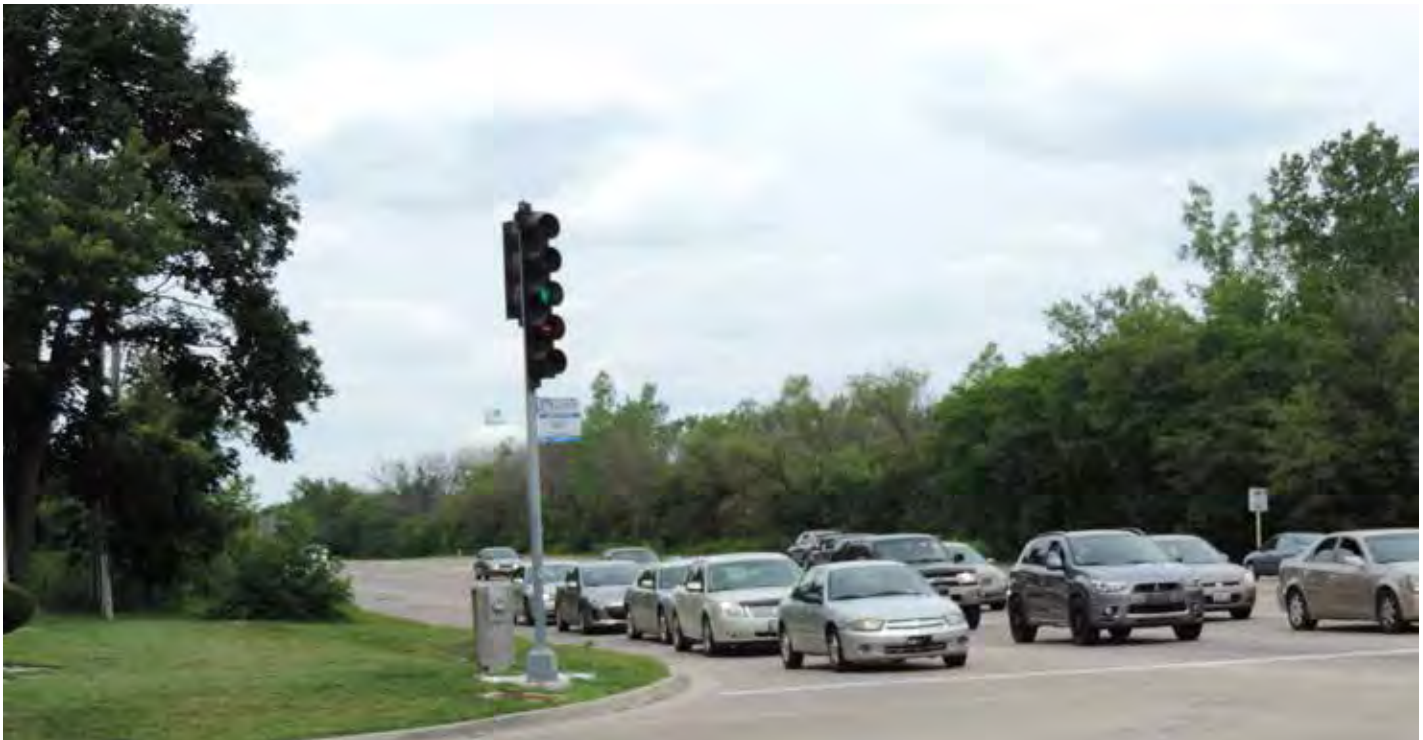
The intersection of Orchard Drive and Route 30 / 211th Street has a Pace bus stop, but no pedestrian crossing markings across the 7 lanes of traffic. Photo by CMAP staff.
